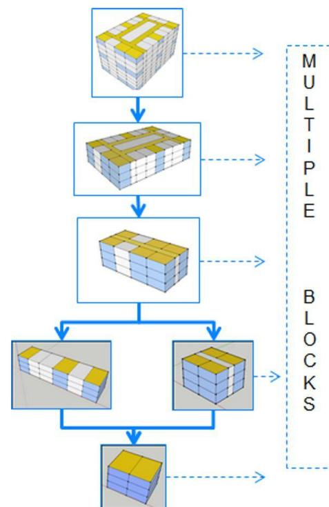
similar to single-family units. To address the building configuration diversity, a dynamic macro structure has been developed within the DOE2.1E model providing an automatic ability to activate/deactivate zones, floors, or surfaces depending on key user inputs on the number of units, number of floors, space types, etc.
